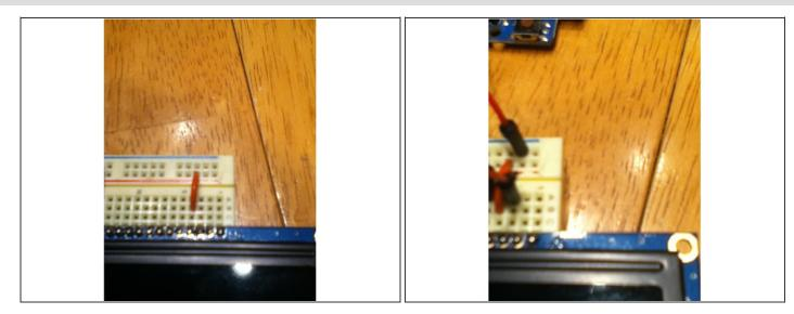
• Connect pin 15 to 5V and then connect either pin 16, 17, or 18 to GND depending on what color you want for your backlight. I picked pin 16 which will make it light up red.
